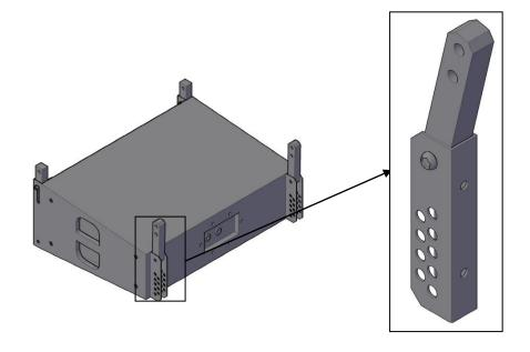
The bracket for the regulation of inclination is in the rear of the case.
