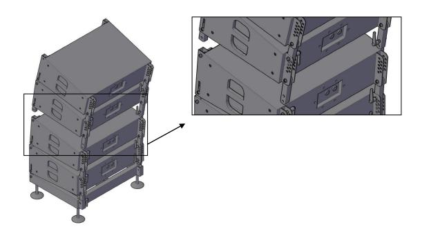
The regulation holes of the bracket allow to choose the desired inclination of the top speaker than the bottom speaker.
