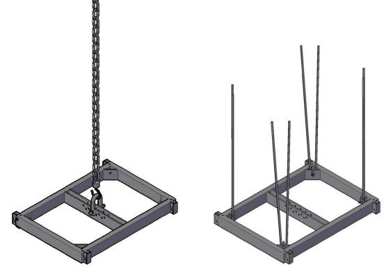
Suspending the bumper from holes for suspension and regulation of inclination, it is possible to determine the inclination of the entire system. Inclination value depends from hole and speakers used because of varying the number of speakers, change the center of gravity, so for an exact operation use an inclinometer.
