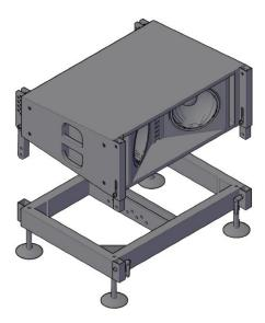
In case of installation in Flying mode, use the bumper without feet, attach the speaker to the sides via connecting bracket, then connect the rear brackets adjusting the inclination.
